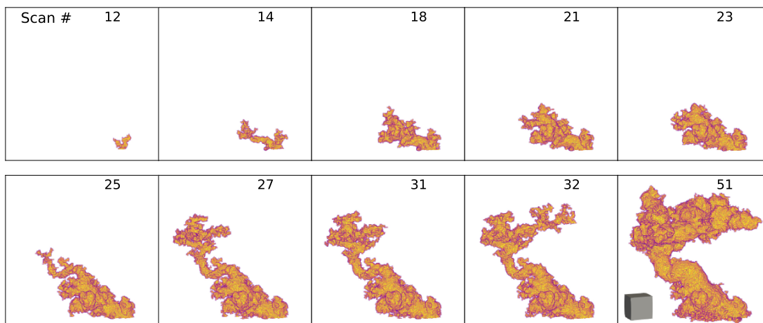
Figure 5.13: Projection of 3D rendering of a conical wormhole at different time instances showing the evolution of the wormhole in acidized PIN44 core. Rendered data is generated by subtracting a tomographic scan from the initial tomographic scan, and visualizing it in TomViz. The sample is half dissolved therefore all the renderings are cropped based on Scan-51 to improve the visualization. To represent the size of wormhole, a scaling cube of 3.4 mm sides is shown in Scan-51.
