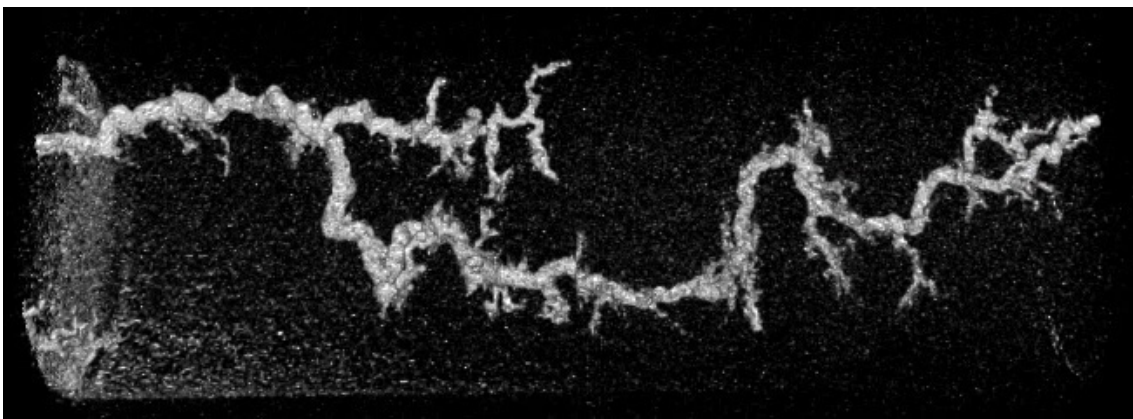
Figure 1.11: A wormhole formed in a lab experiment conducted on Pińczów limestone core with length 11.9 cm and diameter 3.8 cm. The sample is dissolved by HCl solution, which was injected from the left. The data is obtained using an X-ray imaging technique and post-processed to extract the formed channel. [41]
